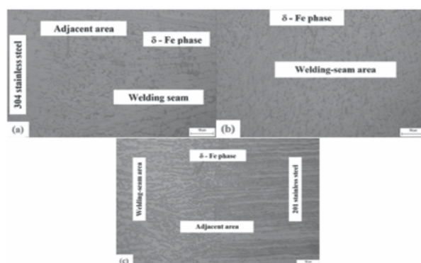
Figure 3. Microstructure of butt welded joint between 304 and 201 stainless steel using GTAW welding process
